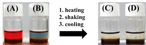
Figure 3. Extraction of Nile Red (A) and indigo (B) from their heptane solutions by PAAPS (the bottom phase). Their concentrations are 3.3 \times 10^{-5} and 0.33 mg/mL, respectively.
